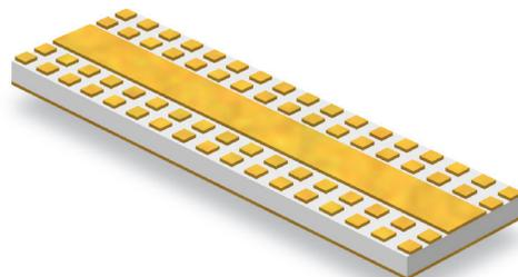
ATP offers build-to-print service for a wide range of materials and metalization schemes. ATP fabricates circuits on substrates from As-Fired Alumina to Beryllium Oxide to Fused Silica, even Silicon. Metalizations range from the standard TaN/TiW/Au to films including Nickel, Palladium, or Titanium.
